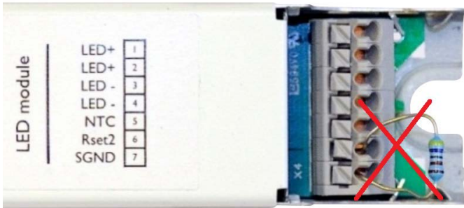
Example of improper use of a non-isolated Rset2 resistor; the bottom lead wire is positioned too close to the driver housing. Contact with the metal driver housing may result in driver malfunctioning or failure.
